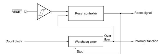
Figure 12-1. Block Diagram of Reset Function
