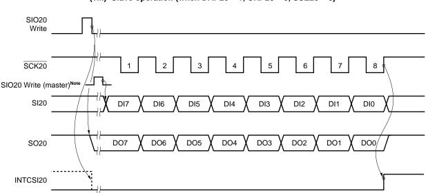
Figure 9-11. 3-Wire Serial I/O Mode Timing (5/7)
