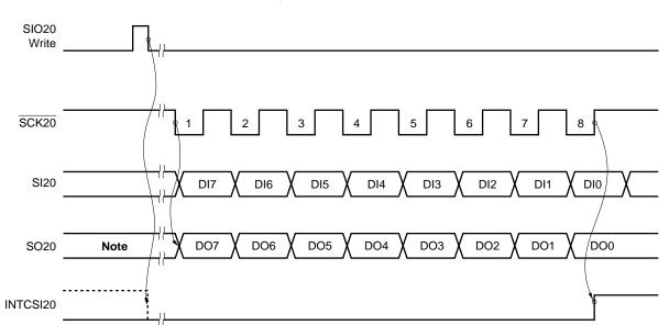
Figure 9-11. 3-Wire Serial I/O Mode Timing (2/7)
