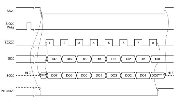
Figure 9-11. 3-Wire Serial I/O Mode Timing (7/7)
