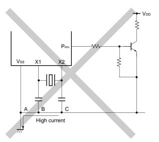
Figure 5-4. Example of Incorrect Resonator Connection (2/2)
