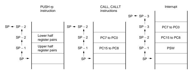
Figure 3-12. Data to Be Saved to Stack Memory
