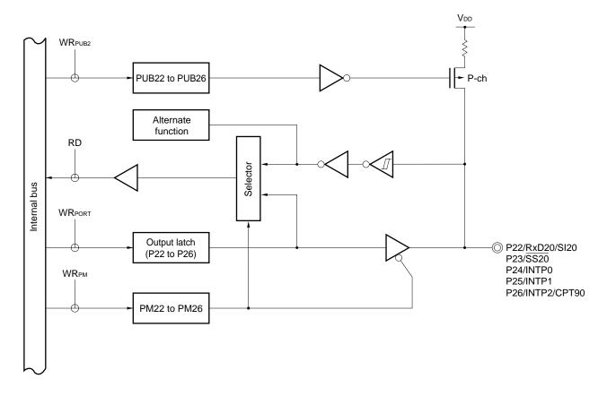
Figure 4-6. Block Diagram of P22 to P26
